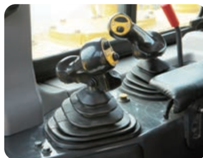
Blade control lever with auto-pitch and new ripper control lever with auto-return function
