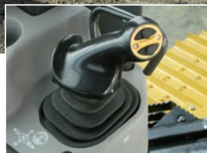
Sistem de control al comenzilor tip Palm (PCCS)
