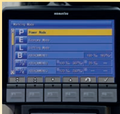
Integrated pressure and flow control system with up to 15 settings to allow maximum effect from attachments.
