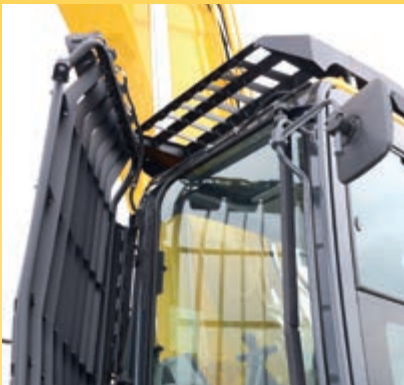
Hinged front guard to allow easy access for windscreen cleaning. The Demolition Safety SpaceCab™ is ROPS compliant with ISO 12117-2:2008.
