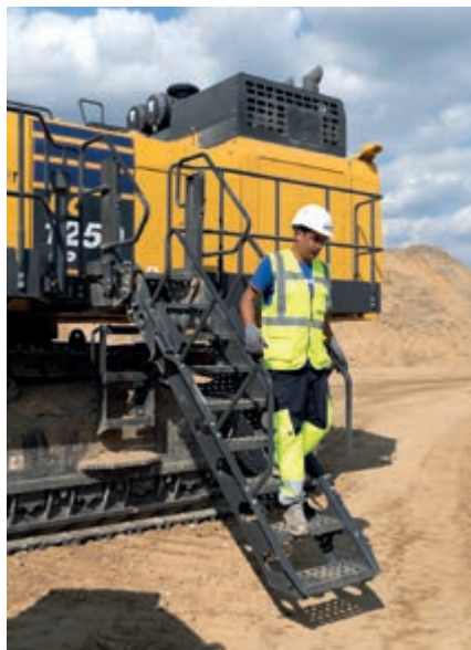
The standard hydraulically operated stairway provides safer access and egress to and from the machine.
