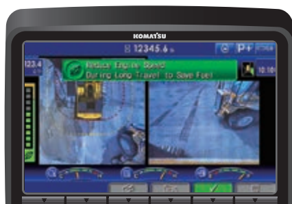
Eco-gauge, Eco guidance and fuel consumption gauge
