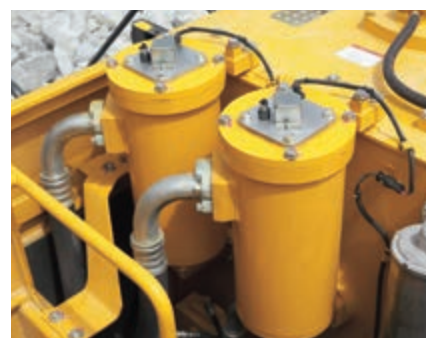
Clogging detector in hydraulic return filter prevents damage of hydraulic system
