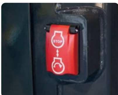
Secondary engine shutdown switch
