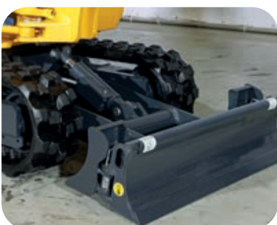
Foldable blade to match the variable undercarriage gauge
