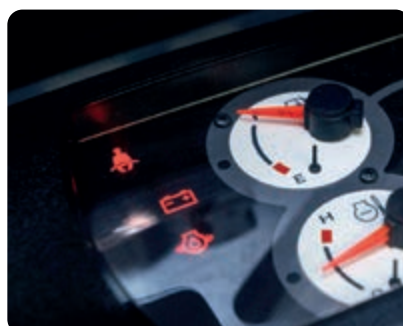
Seat belt caution indicator on the dashboard
