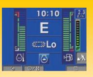
Eco-gauge and fuel consumption gauge further encourage efficient operations
