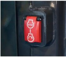
Secondary engine shut down switch
