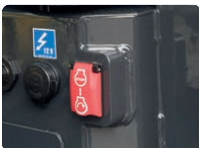
Secondary engine shutdown switch
