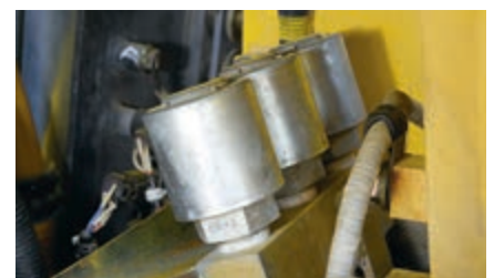
Canister-type breathers facilitate checking and cleaning (optional)
