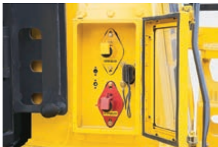
Battery and starter isolator box (optional with mining spec) with jump start receptacle.
