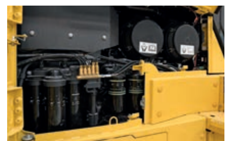
Komatsu designed the D375A-8 with centralised and conveniently located service points to make necessary inspections and maintenance quick and easy.
