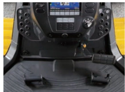
Combined decelerator/brake pedal
