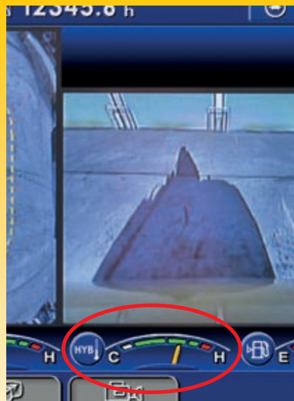
Hybrid system temperature gauge
