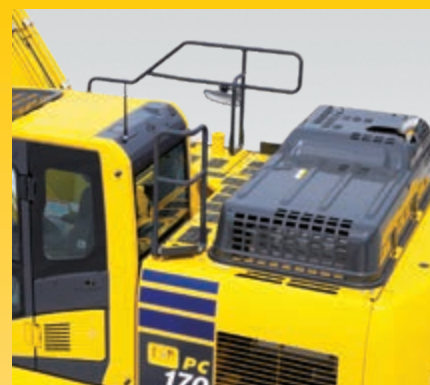
Hand rails and anti-slip plates
