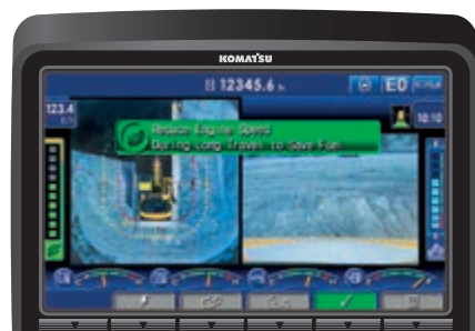
Eco-gauge, Eco guidance and fuel consumption gauge
