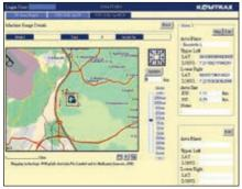
Added security - The "engine lock" feature allows to program when a machine's engine can be started. And with "geo-fence", KOMTRAX<sup>TM</sup> sends notification every time your machine moves in or out of a predetermined operating area.
