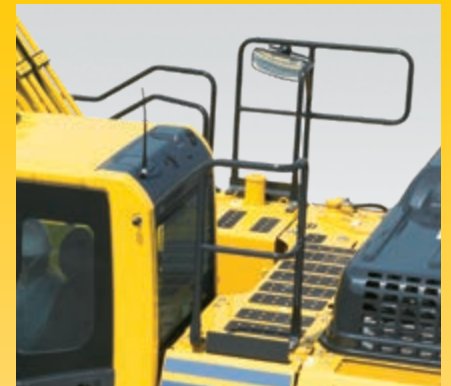
Hand rails and anti-slip plates
