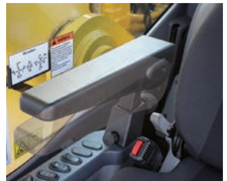
Armrest with simple height adjustment
