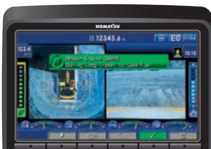
Eco-gauge, Eco guidance and fuel consumption gauge
