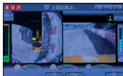
With KomVision, various camera view options are available whilst maintaining constant "birdview" from above the machine
