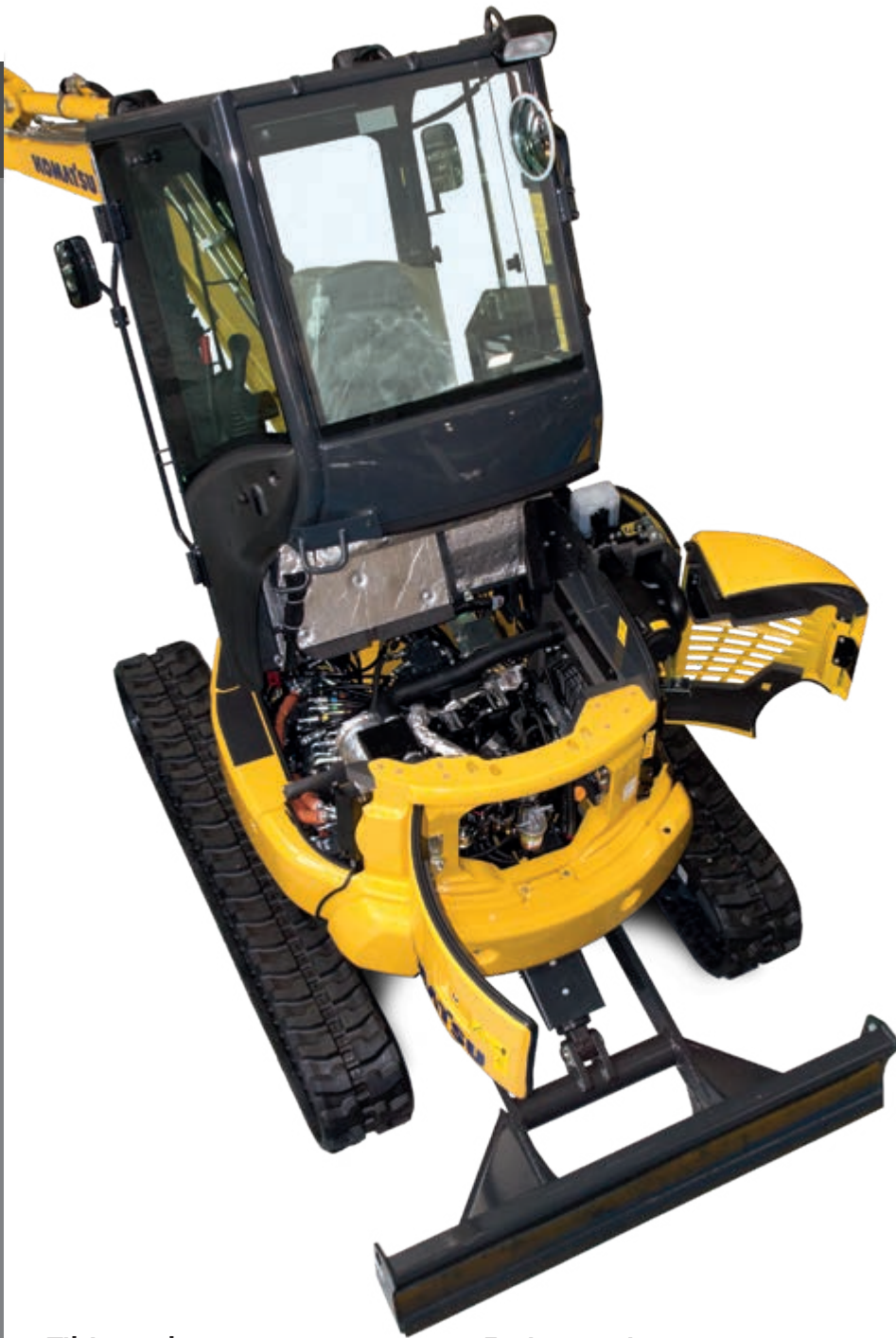
Rear bonnets for quick engine checks, simple inspections, cleaning of the radiators and easy access to the battery
