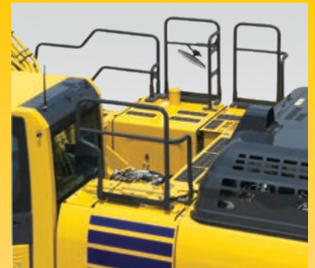
Hand rails and anti-slip plates
