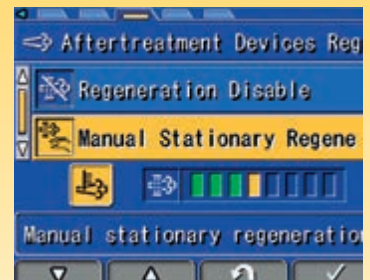
Aftertreatment device regeneration screen for the DPF
