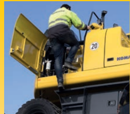
Handrails and anti-slip plates
