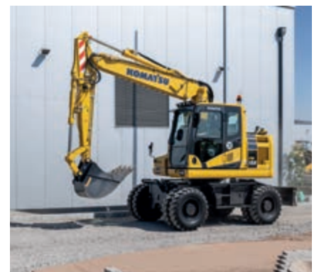
Boom suspension system (ECSS) for increased travel comfort
