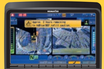
AdBlue® level and refill guidance
