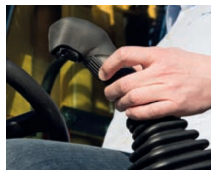
For frequent steering, the Adjustable Joystick Steering option allows to control the machine with less effort
