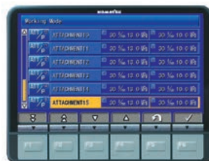
Komatsu Integrated Attachment Control (KIAC)
