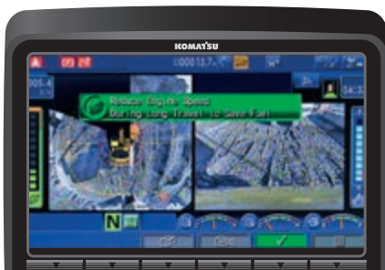
Eco-gauge, Eco guidance and fuel consumption gauge
