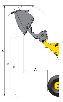
Type B, dump cylinders located outside bucket
