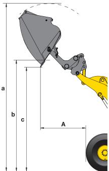
Type B, dump cylinders located outside bucket
