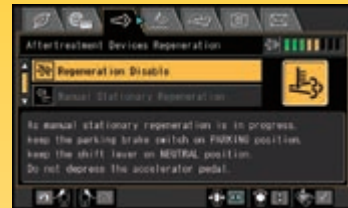
Aftertreatment device regeneration screen for the KDPF
