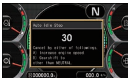
Adjustable auto idle shutdown automatically turns off the engine after it idles for a set period of time
