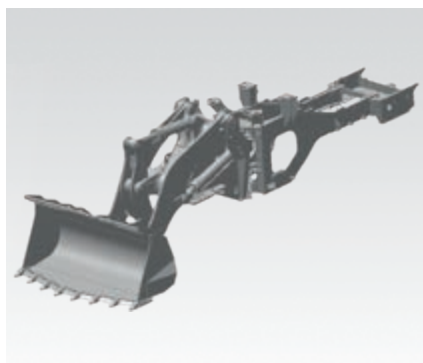
Robust torsion-resistant main frame
