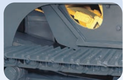
Opening in the crusher side (both sides of undercarriage)
